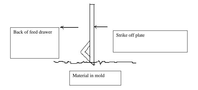
h. Weld 1/8'' - 3/16'' / 3-5mm thick flat bar in staggered heights to the fingers of the agitator. These will act as secondary strike of bars and help the final strike off making a more even pass by limiting the amount of material to strike off.
